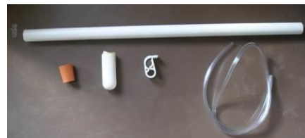
Figure 1. Parts used to build a lysimeter; PVC conduit tube (15mm I.D.), rubber bung, 24mm round end ceramic cup, polycarbonate clamp
